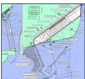
Technical designs for the **Bolham Weir** fish pass, smolt screen and chute are currently undergoing quality assurance with the lead designer. With a restricted land area available for fish pass design, the most cost effective bespoke solution is a super-active baffle fish pass that can be built in the dry through the river bank. The next step is to present the completed design to South West Water and gain support for the SEW team to start the arduous (!) but necessary consenting process.
